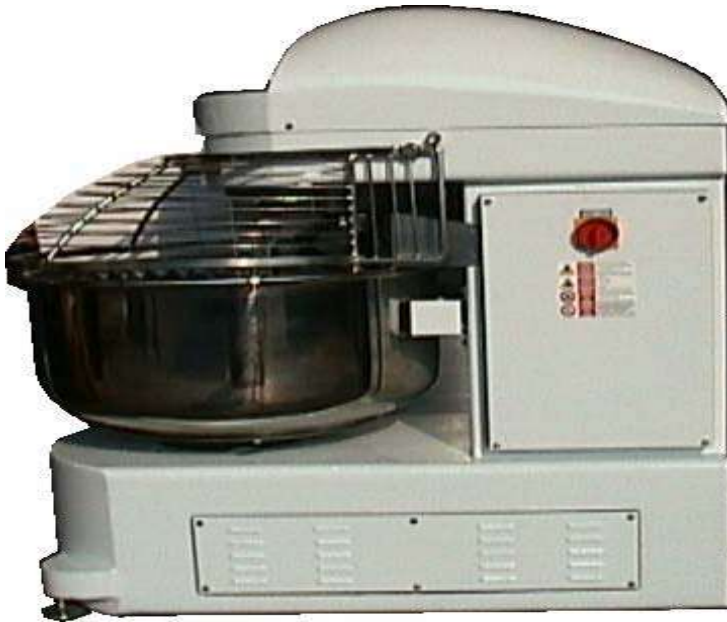
Fig. Fixed and moveable guards
